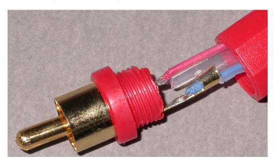
The prepared and tinned DNM Stereo Solid Core speaker cable is shown below.
