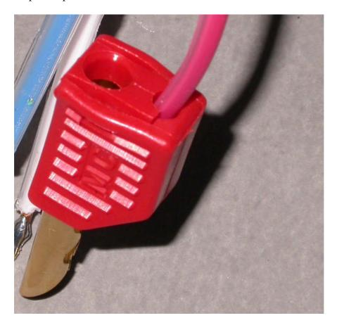
The view below shows how DNM Stereo cable's ideal conductor size allows the 4mm leaf-type plugs to be stacked back-to-back, allowing bi-wiring without the need to solder two conductors into one plug at the amplifier end-- as is normally required when the power amplifier has only one set out output terminals per channel.
