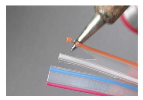
Before it can cool pull off the separated end of the insulation which will slide off easily leaving a clean copper conductor ready to be immediately tinned.
