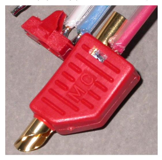
Below is a rear view before the speaker plug cover back is folded closed.
