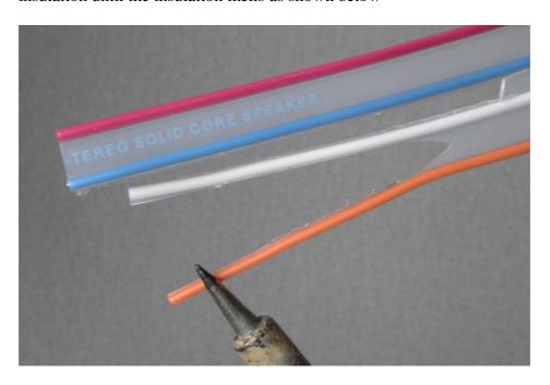
Then immediately apply the soldering iron to the opposite side as shown below
