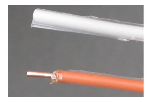
The illustration below shows the DNM Stereo interconnect cable prepared, tinned and ready for the plugs to be fitted.
