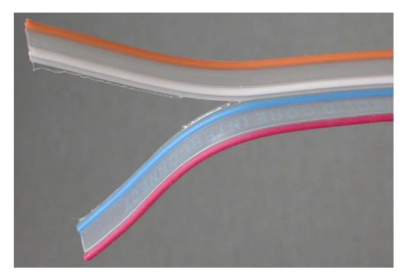
Like the speaker cable, the stereo interconnect conductors are designed to be tear separated from the ribbon, making the cable preparation quick and easy. Again heat is the only sensible way of stripping the insulation from the delicate 0.4mm diameter conductors and it should be applied by heated wire strippers or a soldering iron, as shown for the speaker cable.
