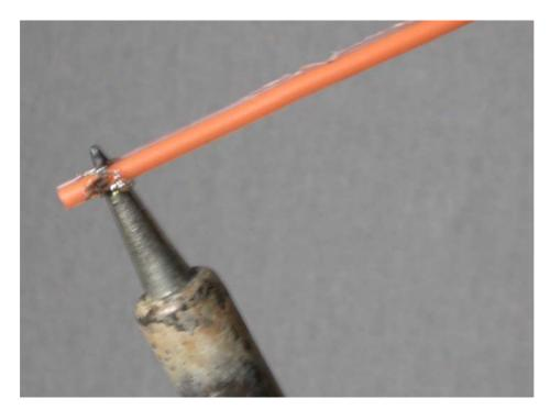
Before it can cool, gently pull the separated insulation which will easily slide off leaving the copper conductor undamaged as shown in the next illustration. Tin the exposed copper immediately before it can oxidise.
