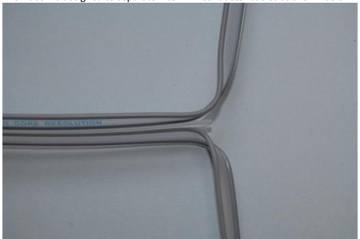
SEPARATE THE RIBBON BY TEARING JUST ENOUGH TO CONNECT THE LEFT AND RIGHT SPEAKERS
