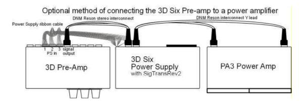
It will be necessary to use a shielded co-axial cable for the pre-amplifier to power-amplifier connection in situations where hum pickup may be likely, as in the case of a valve power amplifier with a high input impedance. This cable can be supplied by DNM Design.
