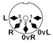
The screen print on the rear panel of the DNM 3D Pre-Amplifier shows the same pattern but does not allocate the ground pin numbers used for the left and right channel. When making up cables with Din plugs for 3D **input and output** connections please follow the connection pattern shown above.
