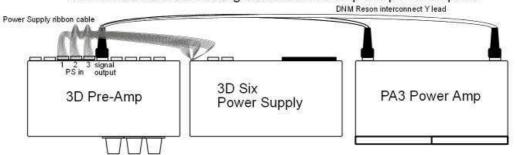
The 3D Twin or Six Pre-Amplifier output signal should normally be connected directly to the power amplifier as shown on page 2. In a system setup where it is more convenient to route the signal via the power supply extra Din sockets are provided on the power supply for this purpose. The power supply must be fitted with "Signal Transfer Board Rev2" (marked in copper on the signal transfer board underneath the power supply motherboard).
